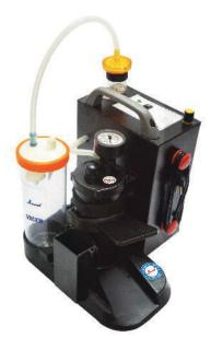
**ASSEMBLY:** AC / DC pump (based on piston system), batteries and PC card are housed in the enclosure. Pedal unit with gauge is attached. The panel has an On / Off switch and four LED lights indicators;
